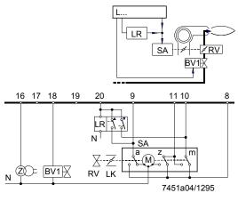
Load control by a modulating controller with galvanically separated control contacts for the positioning directions OPEN or CLOSE.
