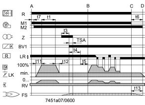
The air damper is kept closed during burner off periods. For other connections, refer to «Connection diagrams».
