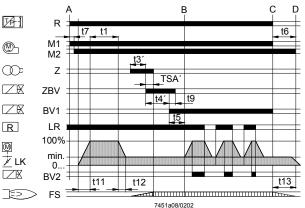
The air damper is kept closed during burner off periods. For other connections, refer to «Connection diagrams».
