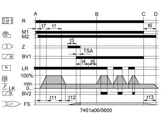
Control of actuator «SA» according to the single-wire principle (actuator «SA»: E.g. SQN3... according to Data Sheet N7808). For other connections, refer to «Connection diagrams».
