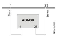
If the mains cables (L-N) are switched, the AGM30 simulates a flame signal (extraneous light). The burner initiates lockout.
