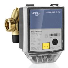
The flow sensor ULTRAHEAT Flow T150 is an ultrasonic volume measurement component for separately approved calculators and open systems. The T150 uses a fast pulse output. Its mechanical features are the same as the ULTRAHEAT T550. Available models have ratings between qp 0.6 and qp 60 and a nominal pressure of up to PN25.
