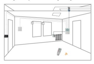
Chilled/heated ceilings (or radiators) via ON/OFF or modulating control outputs:
