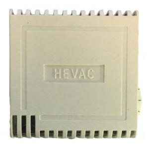
The SRT-DSP is an adjustable setpoint room sensor that is intended for use with Hevac brand HTC 3, 5 and Digital series controllers. The sensor has a NTC characteristic (increase in temperature = decrease in resistance) and changes approximately 80 ohms per degree. Both a concealed and exposed adjustment knob are included, allowing plus or minus 3.5°C from the HTC's main setpoint.
